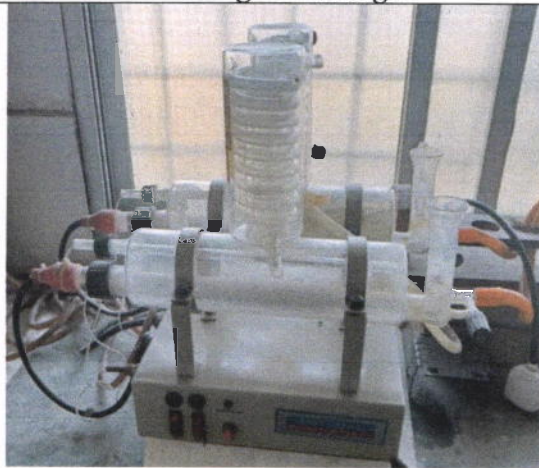
Eco still Distillation Assembly
